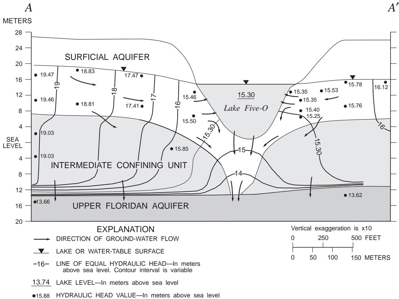
**Figure 10.** Hydrogeologic section A-A' through Lake Five-O, showing vertical head distribution near the lake for January 17, 1990. (Location of section is shown in fig. 3.)
