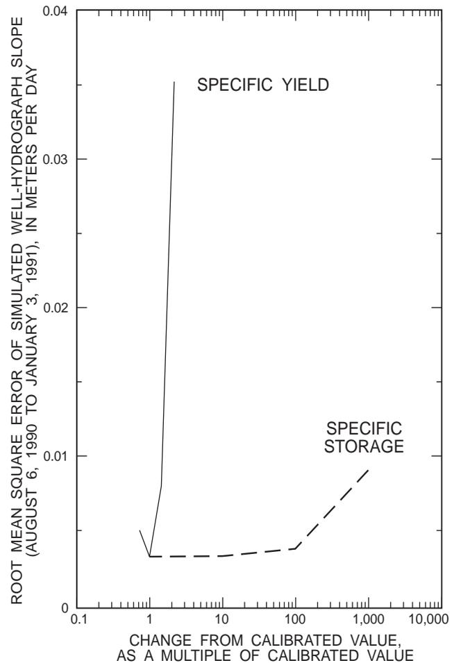
**Figure 19.** Sensitivity of transient model of the ground-water flow system near Lake Five-O to changes in aquifer storage properties.
