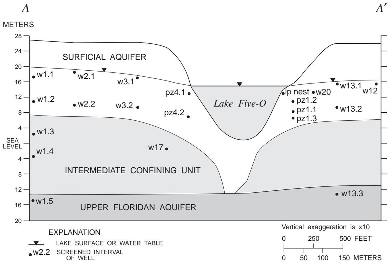
**Figure 4.** Hydrogeologic section A-A' through Lake Five-O showing midpoints of screened intervals of observation wells used to construct the section. (Location of section is shown in figure 3. Hydrogeologic section A-A' revised from Andrews and others, 1990.)
