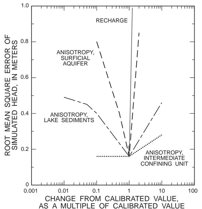
**Figure 18.** Sensitivity of steady-state models of ground-water flow system near Lake Five-O to changes in recharge and anisotropy.
