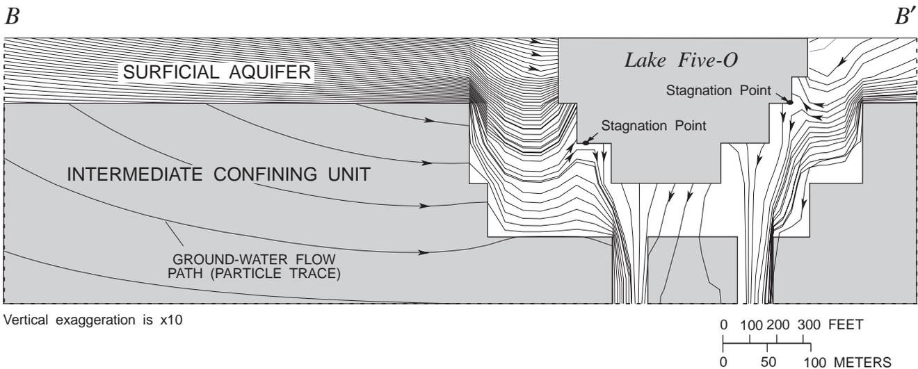
**Figure 23.** Particle traces projected onto hydrogeologic-section B-B' near Lake Five-O.
