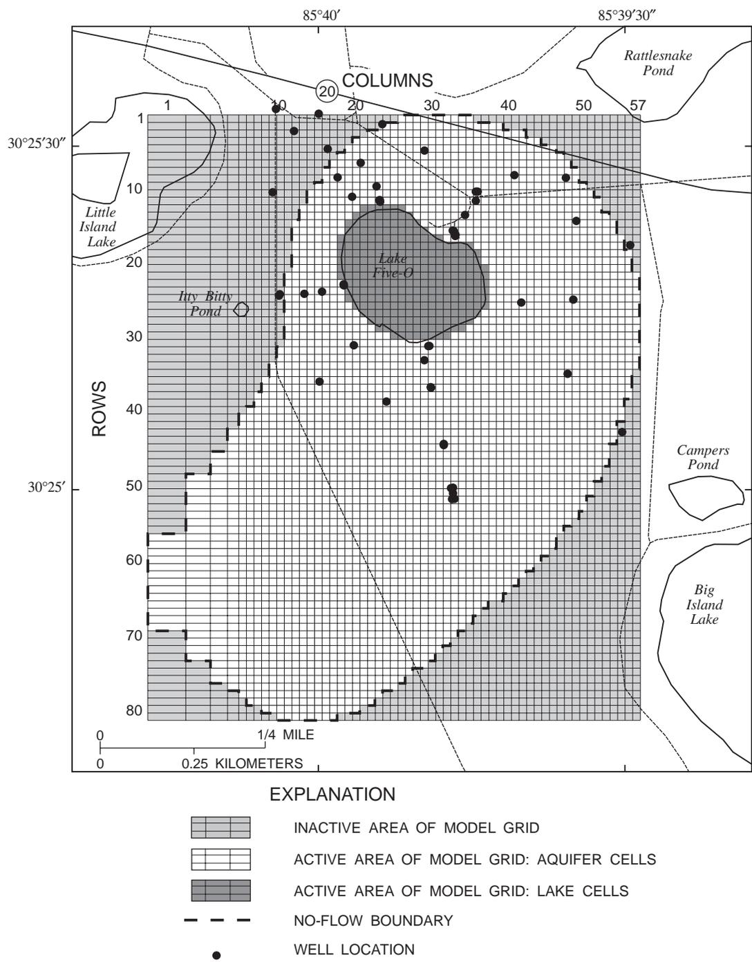
**Figure 14.** Areal discretization and boundary conditions for simulation models of the ground-water flow system near Lake Five-O.
