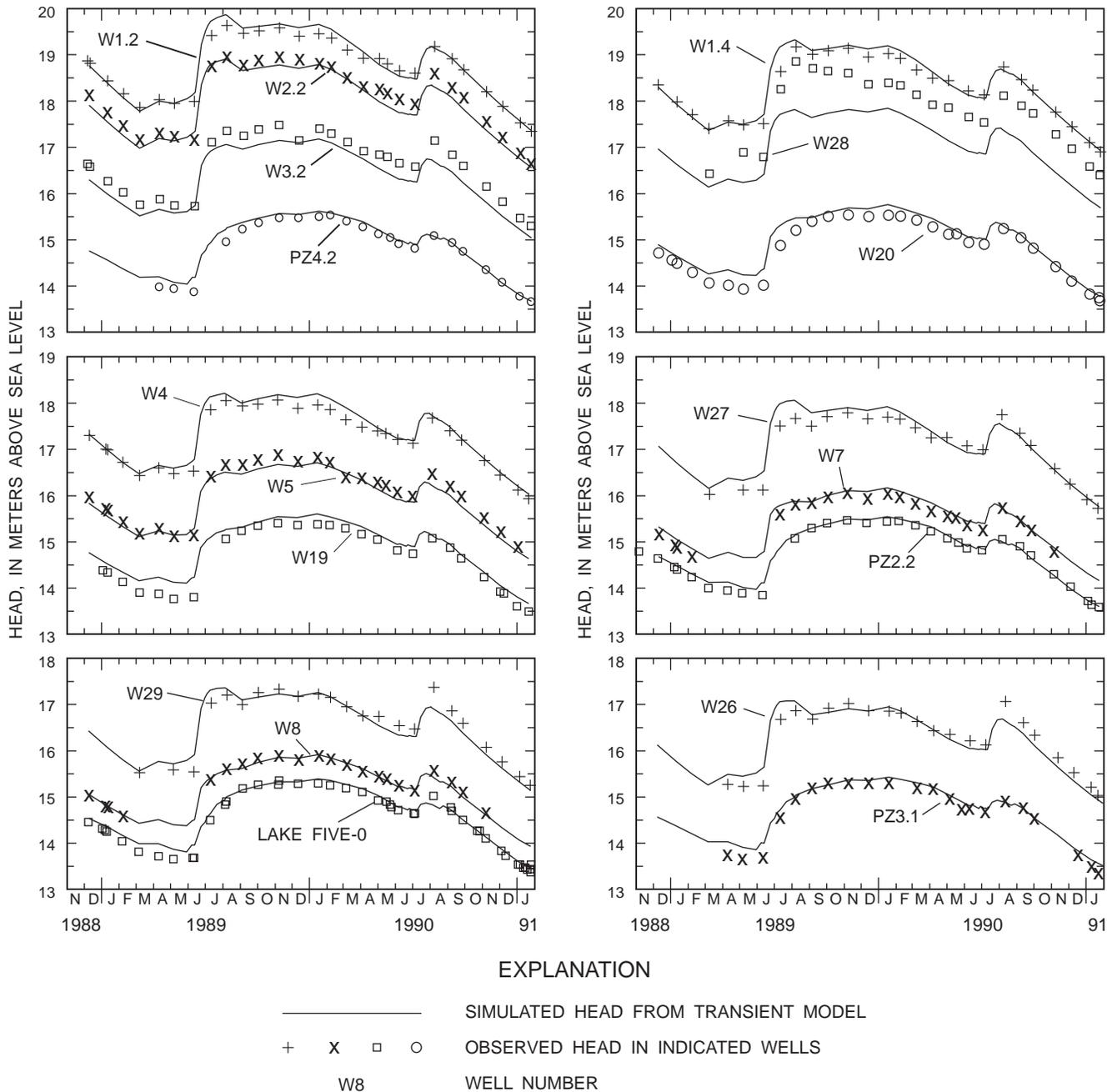
**Figure 20.** Simulated and observed heads for Lake Five-O and adjacent ground-water system, December 12, 1988, through January 22, 1991.
