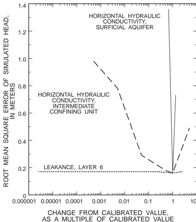
**Figure 17.** Sensitivity of steady-state models of ground-water flow system near Lake Five-O to changes in horizontal hydraulic conductivity and leakance of layer 6.
