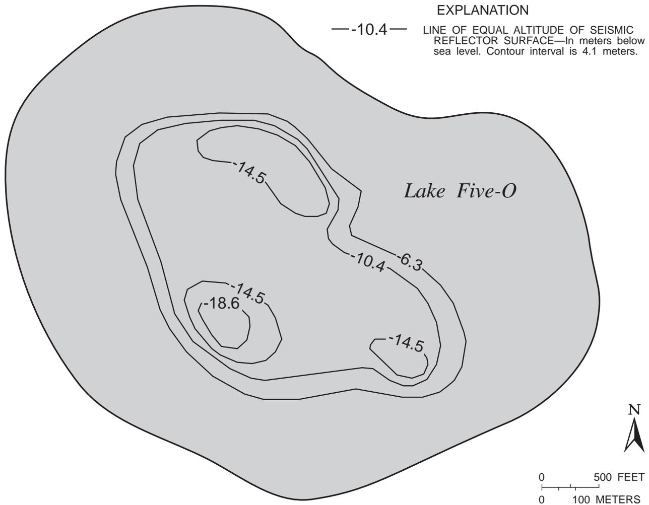
**Figure 5.** Altitude of seismic reflector surface beneath Lake Five-O. (Hal Davis, U.S. Geological Survey, written commun., 1991.)
