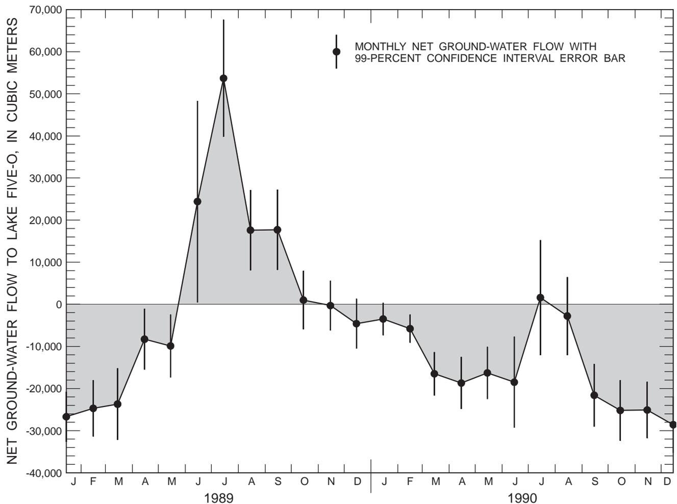
**Figure 12.** Computed monthly net ground-water flow to Lake Five-O during 1989-90.
