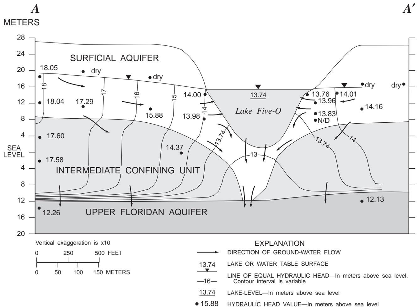
**Figure 9.** Hydrogeologic section A-A' through Lake Five-O, showing vertical head distribution near the lake for April 13, 1989. (Location of section is shown in fig. 3).
