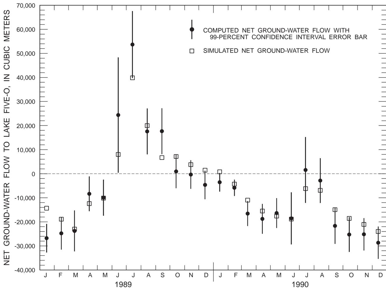
Figure 21. Simulated and computed monthly net ground-water flow to Lake Five-O, 1989-90.
