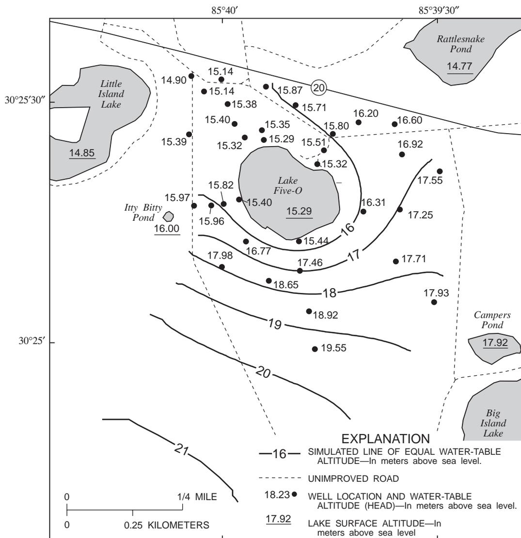
Figure 16. Simulated and observed water levels in the surficial aquifer near Lake Five-O, October 4, 1989.
