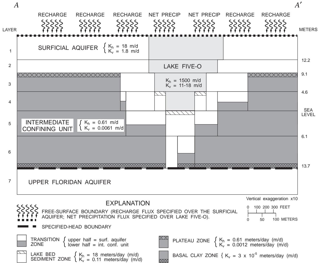
**Figure 15.** Vertical discretization, boundary conditions, and calibrated values of hydraulic conductivity for simulation models of the ground-water flow system near Lake Five-O.
