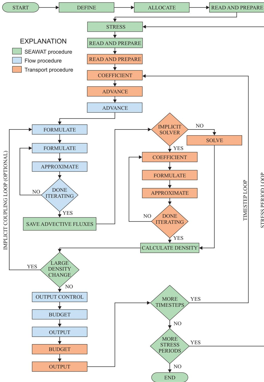
Figure 7. Step-by-step procedures of the SEAWAT program.
