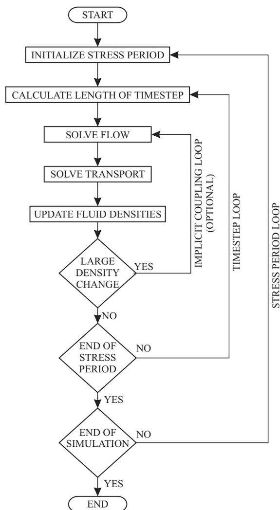
**Figure 4.** Generalized flow chart of the SEAWAT program.
